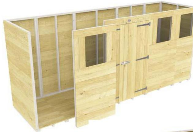
**11a.** Place the final front panel as shown (Below) to complete the outer framework. Then adjust and screw down the panels to the shed floor to make the build secure. This requires an extra 3x Screws.
