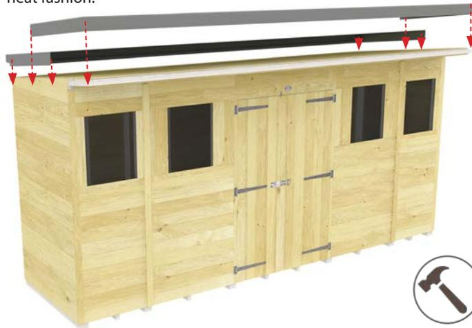
**18c.** Trim down excess felt with a stanley knife. Remember to overlay the 1st felt to avoid rain leaks.
