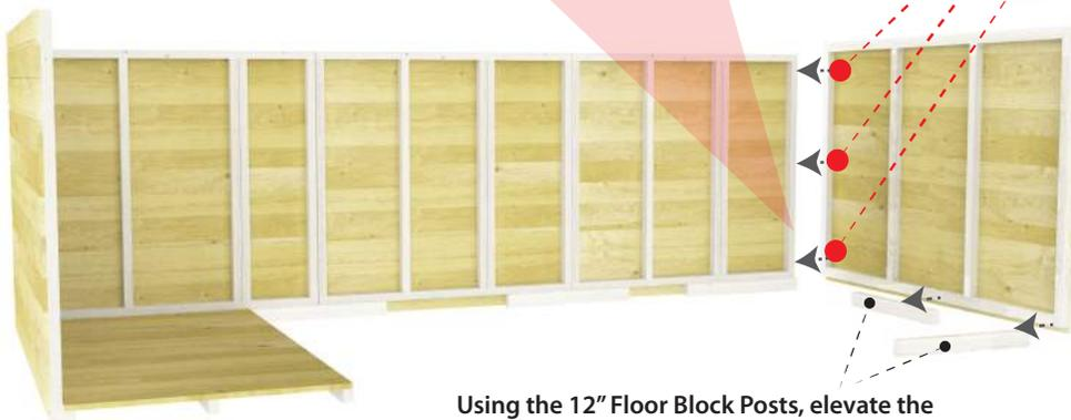
Using the 12" Floor Block Posts, elevate the right side panel and screw in sides to secure against the 3rd back panel side post as shown.
