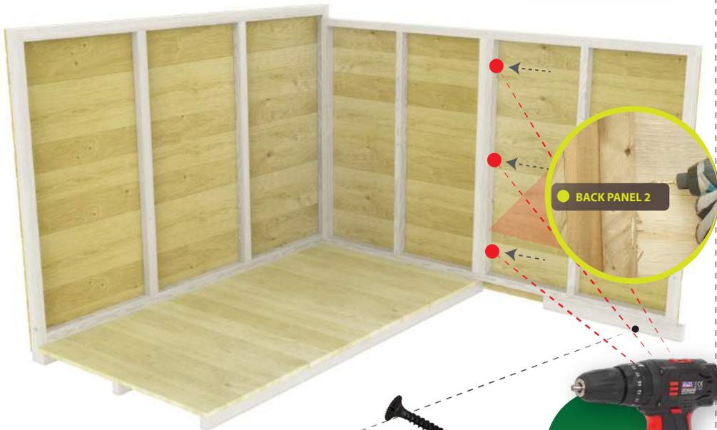
Use a 12" Floor Block Posts elevate the 2nd back panel and screw in sides to secure againsts the 1st back panel side post as shown.
