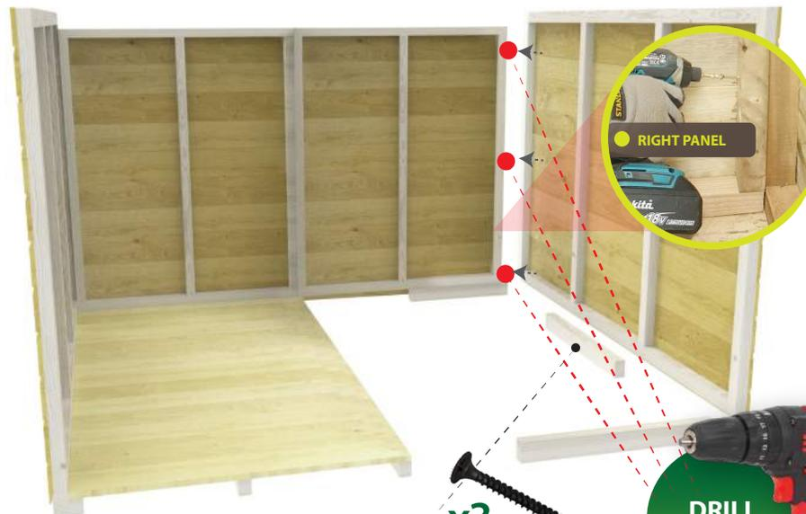
Use 12" Floor Block Posts elevate the right side panel and screw in sides to secure againsts the 2nd back panel side post as shown.
