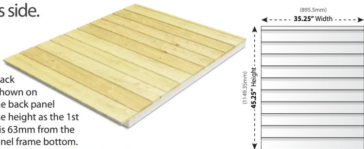
Position the 2nd back panel in place as shown on diagram below. The back panel 2 must be the same height as the 1st back panel which is 63mm from the ground to back panel frame bottom.
